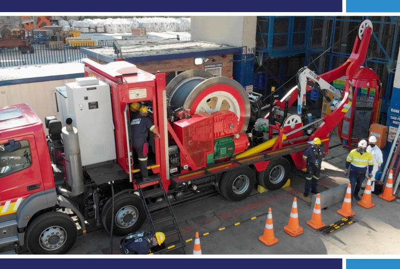
Our truck-mounted Mobile Mine Rescue Hoists (MMRHs) are designed to address the urgent need for rapid response and resolution to underground mining emergencies and safety incidents. Engineered with safety and operators in mind, our MMRWs are fully roadworthy and self-powered, with patented hydraulics and hoist technology, allowing rescue teams to respond faster, mitigate risk of death, and reduce mine downtime.
